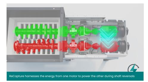
Developed by the M&J's expert engineers, ReCapture intelligently harnesses the energy from one motor to power the other during shaft reversals, contributing up to 25% in energy savings of M&J e-drive – validated through on-site testing.
